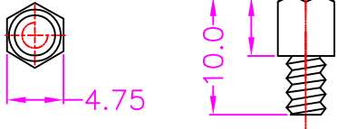
#4-40UNC SCREWLOCK INSTALLED
